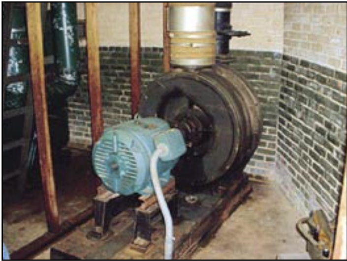
The 100" Compressor for the Grand Ophicleide, Tuba Imperial, Tuba Maxima, and Tuba Mirabilis.
