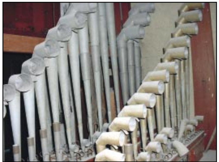
Some pipes of the Trumpet Mirabilis broken at the necks by careless workmen while hanging plastic sheeting on the inside of the grill prior to painting the outside of the grill.
