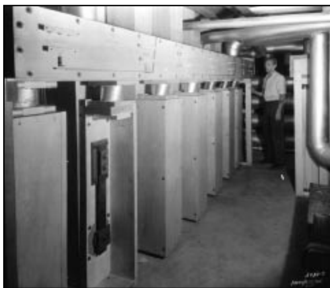
Boots of the DDDDD to GGGGG# pipes. The cover has been removed from the DDDDD# boot to reveal the massive tone-producing mechanism within.
